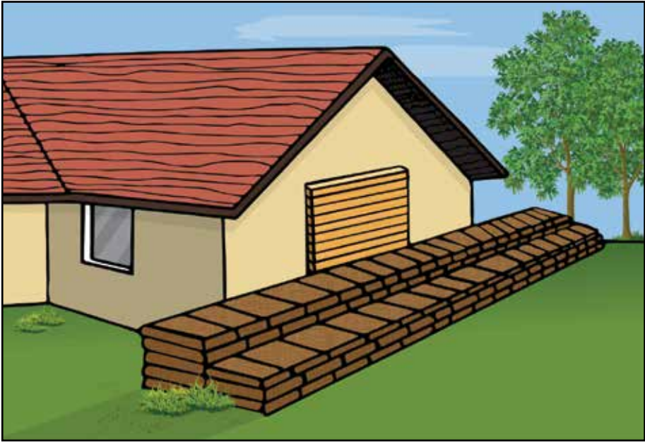
Fig. 5 - Sandbag Stacking Against Buildings
