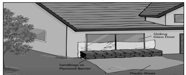
Fig. 11 SLIDING GLASS DOOR SEALING Control of flows to prevent seeping around sliding glass doors.
