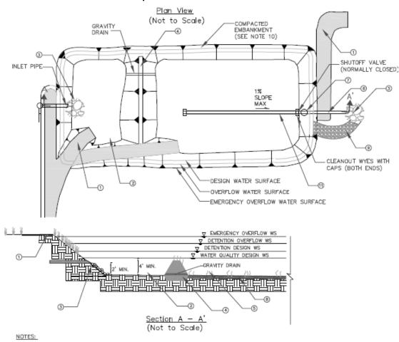
Figure 2 Example Infiltration Basin Schematic
