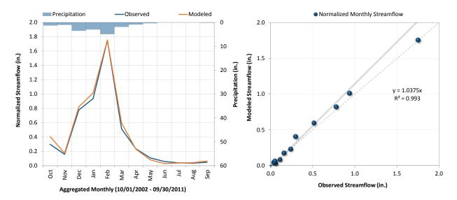
Figure C-1- 12. Average monthly flow at Brea Creek below Brea Dam, near Fullerton, CA (Station ID: 11088500).
