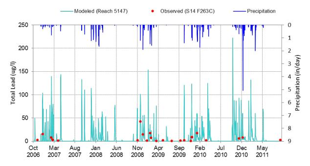
Figure C-1-43. Simulated vs. observed timeseries plots for Total Lead (10/1/2006 through 9/30/2011) at San Gabriel River Mass Emission Station (S14).
