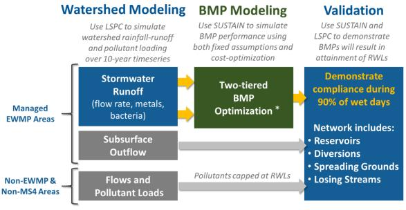
\* Tier 1: Cost-optimize load reduction of limiting pollutant for each subwatershed (end-of-pipe)
