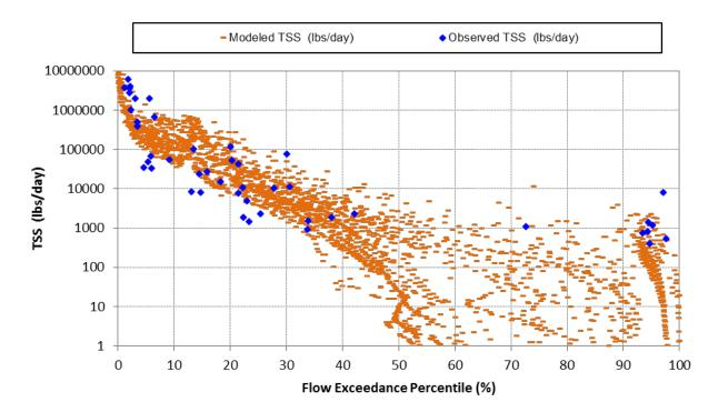
Figure C-1-36. Simulated vs. observed load duration plots for Total Sediment (10/1/2006 through 9/30/2011) at San Gabriel River Mass Emission Station (S14).
