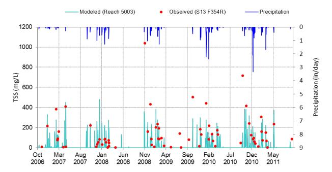
Figure C-1-24. Simulated vs. observed timeseries plots for Total Sediment (10/1/2006 through 9/30/2011) at Coyote Creek Mass Emission Station (S13).
