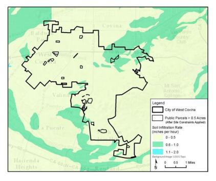
Figure E-9 Soil Infiltration Rates
