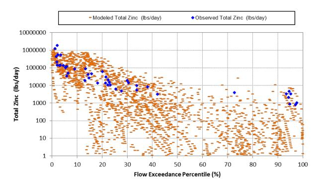
Figure C-1-38. Simulated vs. observed load duration plots for Total Zinc (10/1/2006 through 9/30/2011) at San Gabriel River Mass Emission Station (S14).
