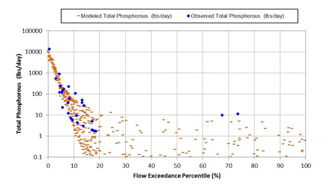
Figure C-1-33 Simulated vs. observed load duration plots for Total Phosphorous (10/1/2006 through 9/30/2011) at Coyote Creek Mass Emission Station (S13).
