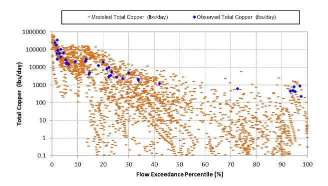
Figure C-1-40. Simulated vs. observed load duration plots for Total Copper (10/1/2006 through 9/30/2011) at San Gabriel River Mass Emission Station (S14).
