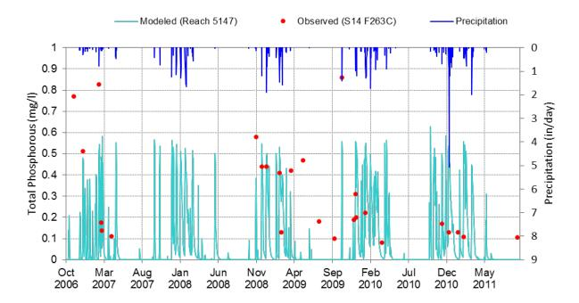
Figure C-1-45. Simulated vs. observed timeseries plots for Total Phosphorous (10/1/2006 through 9/30/2011) at San Gabriel River Mass Emission Station (S14).
