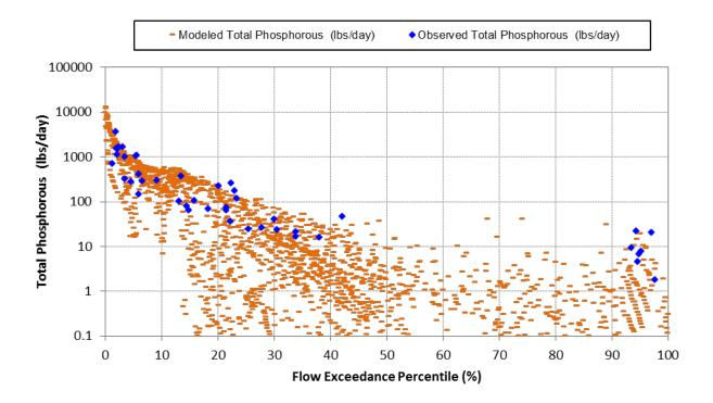
Figure C-1-44 Simulated vs. observed load duration plots for Total Phosphorous (10/1/2006 through 9/30/2011) at San Gabriel River Mass Emission Station (S14).
