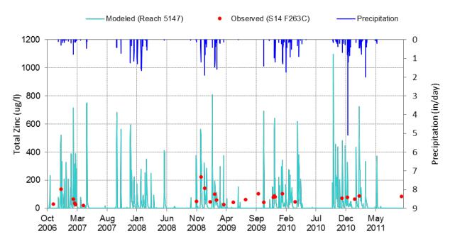
Figure C-1-39. Simulated vs. observed timeseries plots for Total Zinc (10/1/2006 through 9/30/2011) at San Gabriel River Mass Emission Station (S14).
