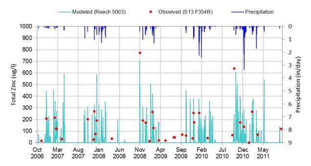
Figure C-1-26. Simulated vs. observed timeseries plots for Total Zinc (10/1/2006 through 9/30/2011) at Coyote Creek Mass Emission Station (S13).
