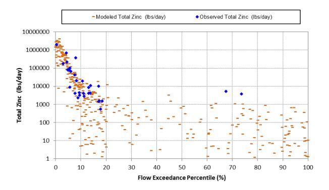
Figure C-1-25. Simulated vs. observed load duration plots for Total Zinc (10/1/2006 through 9/30/2011) at Coyote Creek Mass Emission Station (S13).
