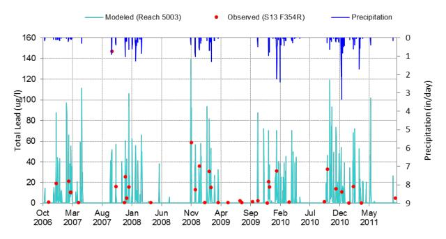
Figure C-1-30. Simulated vs. observed timeseries plots for Total Lead (10/1/2006 through 9/30/2011) at Coyote Creek Mass Emission Station (S13).
