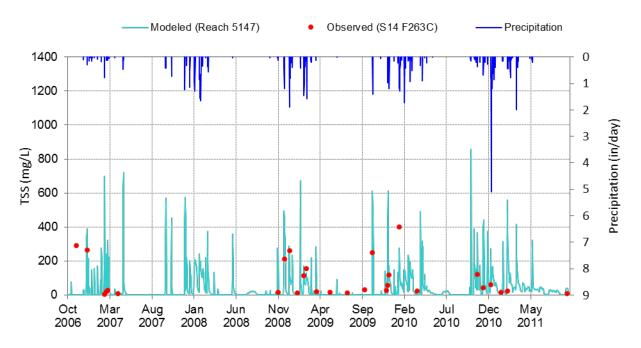
Figure C-1-37. Simulated vs. observed timeseries plots for Total Sediment (10/1/2006 through 9/30/2011) at San Gabriel River Mass Emission Station (S14).
