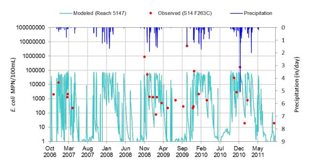
Figure C-1-46. Simulated vs. observed timeseries plots for *E. coli* (10/1/2006 through 9/30/2011) at San Gabriel River Mass Emission Station (S14).
