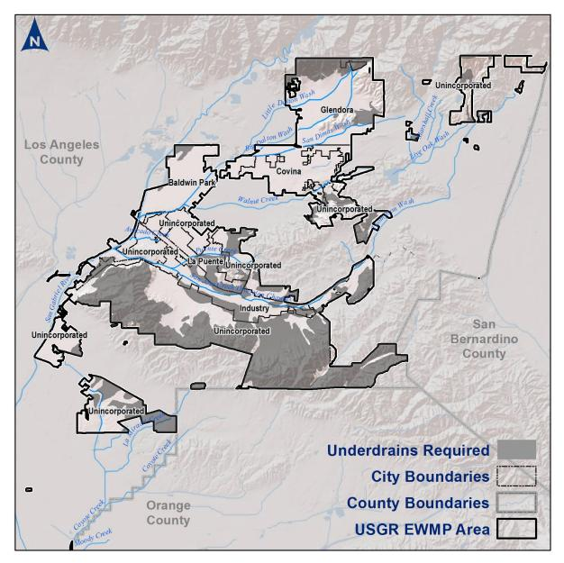
Figure C-3-6. Areas where underdrains will likely be required (e.g. where subsoil infiltration rates are estimated less than 0.3 in/hr)
