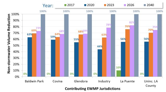
Figure 3-1. Schedule for Non-stormwater Reductions via Implementation of EWMP Structural BMPs
