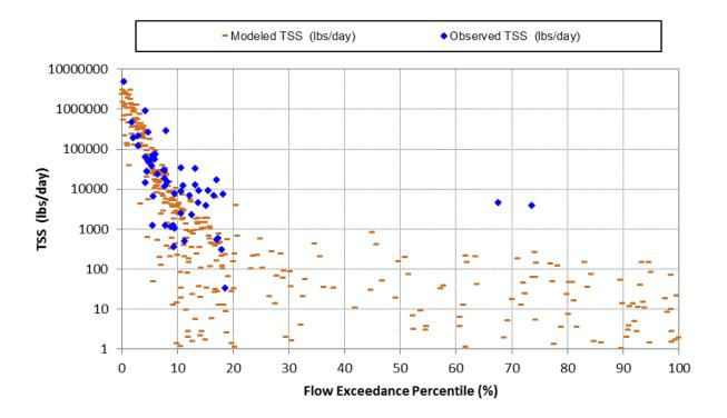
Figure C-1-23. Simulated vs. observed load duration plots for Total Sediment (10/1/2006 through 9/30/2011) at Coyote Creek Mass Emission Station (S13).
