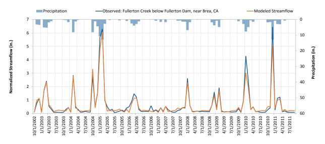
Figure C-1- 9. Monthly flow at Fullerton Creek below Fullerton Dam, near Brea, CA (Station ID: 11089500).
