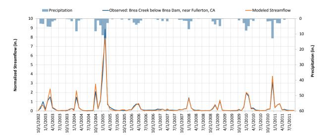
Figure C-1- 11. Monthly flow at Brea Creek below Brea Dam, near Fullerton, CA (Station ID: 11088500).
