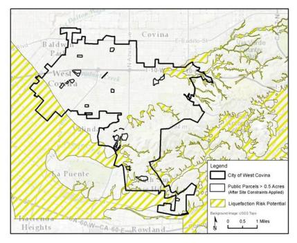
Figure E-11 High Liquefaction Potential
