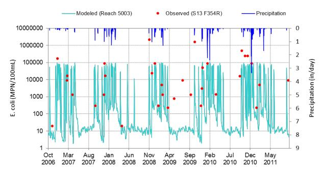
Figure C-1-35. Simulated vs. observed timeseries plots for *E. coli* (10/1/2006 through 9/30/2011) at Coyote Creek Mass Emission Station (S13).
