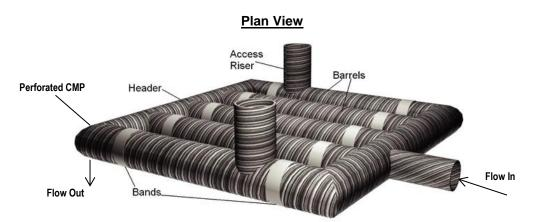
Figure 3 Conceptual Subsurface Infiltration Using CMP (modified from Contech, 2015)
