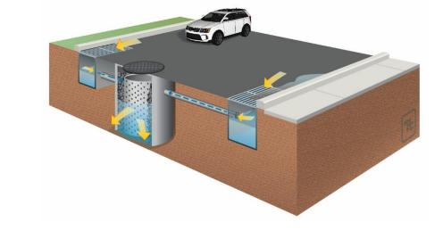
Figure B-2-9. Typical distributed infiltration BMP schematic showing perforated concrete dry well variation (arrows indicate water pathways; for infiltration trenches, see Figure B-2-6 and omit vegetation).
