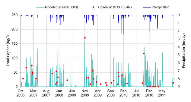
Figure C-1-28. Simulated vs. observed timeseries plots for Total Copper (10/1/2006 through 9/30/2011) at Coyote Creek Mass Emission Station (S13).
