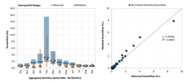
Figure C-1-4. Monthly flow interquartiles at Brea Creek below Brea Dam, near Fullerton, CA (Station ID: 11088500).
