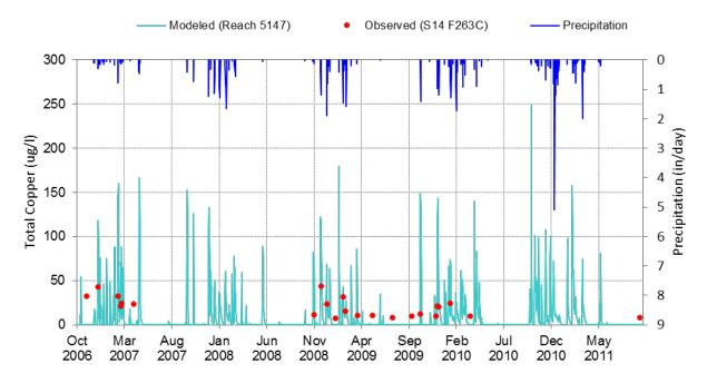
Figure C-1-41. Simulated vs. observed timeseries plots for Total Copper (10/1/2006 through 9/30/2011) at San Gabriel River Mass Emission Station (S14).
