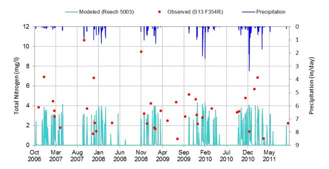
Figure C-1-32. Simulated vs. observed timeseries plots for Total Nitrogen (10/1/2006 through 9/30/2011) at Coyote Creek Mass Emission Station (S13).
