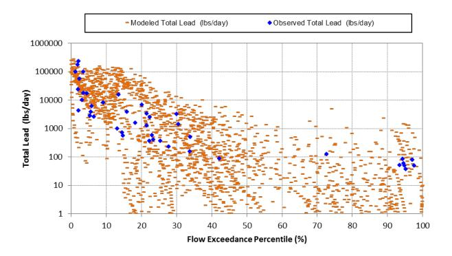
Figure C-1-42 Simulated vs. observed load duration plots for Total Lead (10/1/2006 through 9/30/2011) at San Gabriel River Mass Emission Station (S14).
