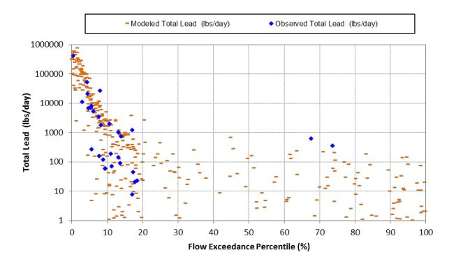
Figure C-1-29 Simulated vs. observed load duration plots for Total Lead (10/1/2006 through 9/30/2011) at Coyote Creek Mass Emission Station (S13).
