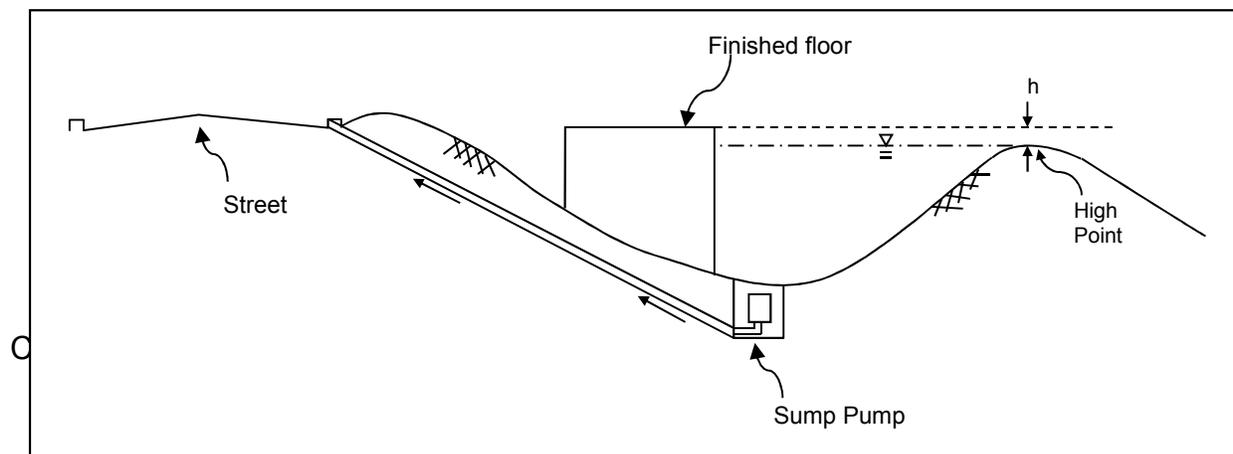
The finished floor elevation of the proposed project is below the sump overflow elevation, such as a condo complex with subterranean parking.
