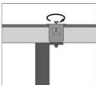
**Step 3.** Tighten the hex bolt using 7/16" socket and torque to 55 in.-Lbs, to secure PV module.
