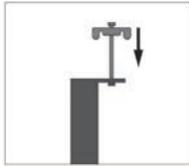
**Step 1.** Insert the conductive mid clamp, each consisting of (1) conductive mid clamp, (1) lock washer, and (1) hex bolt, or (1) serrated hex bolt into the 1/4" diameter attachment hole in both high and low brackets that are holding an existing PV panel. (Do not tighten the hex bolt, but provide 2 turns to ensure that the bolt stays in place.)
