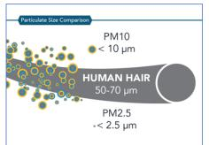
deposition on the filter 'tape', measurement with beta rays, and movement of the filter tape. PM<sub>10</sub> and PM<sub>2.5</sub> are the most common particulate sizes to be measured by both methods and are presented relative to the size of a human hair (see insert). All PM<sub>10</sub> data included in this analysis are from BAM instruments. Thus, no instrument corrections or instrument to instrument comparisons are discussed in this report.
