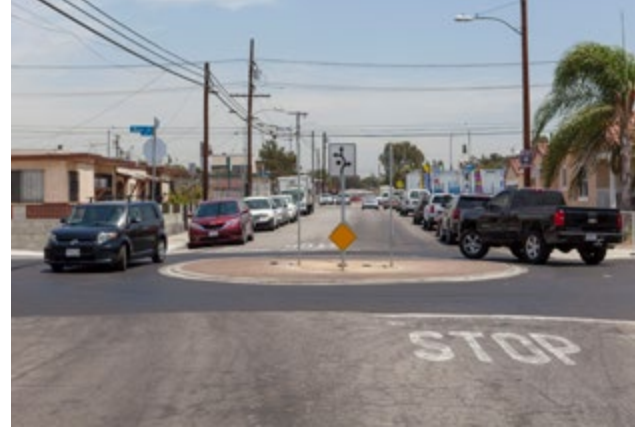
Traffic Circles and Roundabouts are intersection designs that can reduce vehicle speeds and conflicts.
