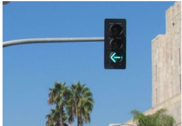
Left Turn Signal Phasing provides a green arrow for left turning vehicles while stopping conflicting vehicles and pedestrians.
