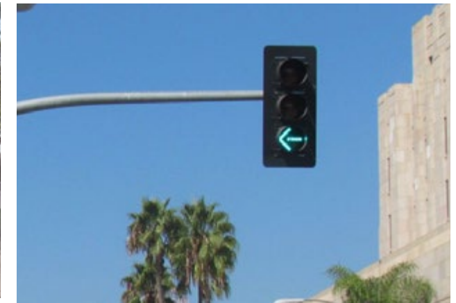
Left Turn Signal Phasing provides a green arrow for left turning vehicles while stopping conflicting vehicles and pedestrians.
