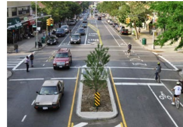
Roadway Reconfigurations typically reduce the number of vehicular travel lanes and may reallocate space to pedestrians and bicyclists and allow room for vehicle turning lanes. Narrower traffic lanes may also contribute to slower speeds while the addition of street trees along corridors can have a traffic calming effect.
