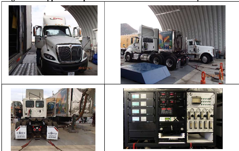
Figure 2-1. Typical Setup of Test Vehicles on the Chassis Dynamometer
