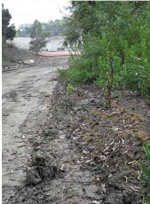
Photo 4: Photo taken from Photo Point 3 depicting orange rusty redoximorphic features on the surface of soils along the banks of the road (on the right). This was typical in areas throughout the reservoir.
