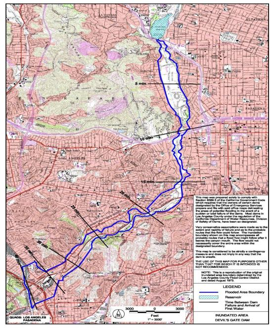
Figure 3 Arroyo Seco Dam Failure Inundated Area
