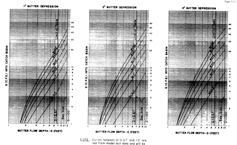
model test data are available. CURB OPENING CATCH BASIN CAPACITIES
