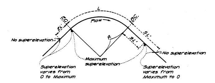
When determining superelevated water surfaces for freeboard (See Section C-4 for Freeboard) without easement curves, begin the surface change at a point 5 L' downstream of the B.C. of curve with no superelevation, taper to maximum superelevation at a point 3 L' downstream of the B.C. of curve, carry maximum superelevation to the E.C. of curve, and taper to no superelevation at a point 2 L' upstream of the E.C. DAC
