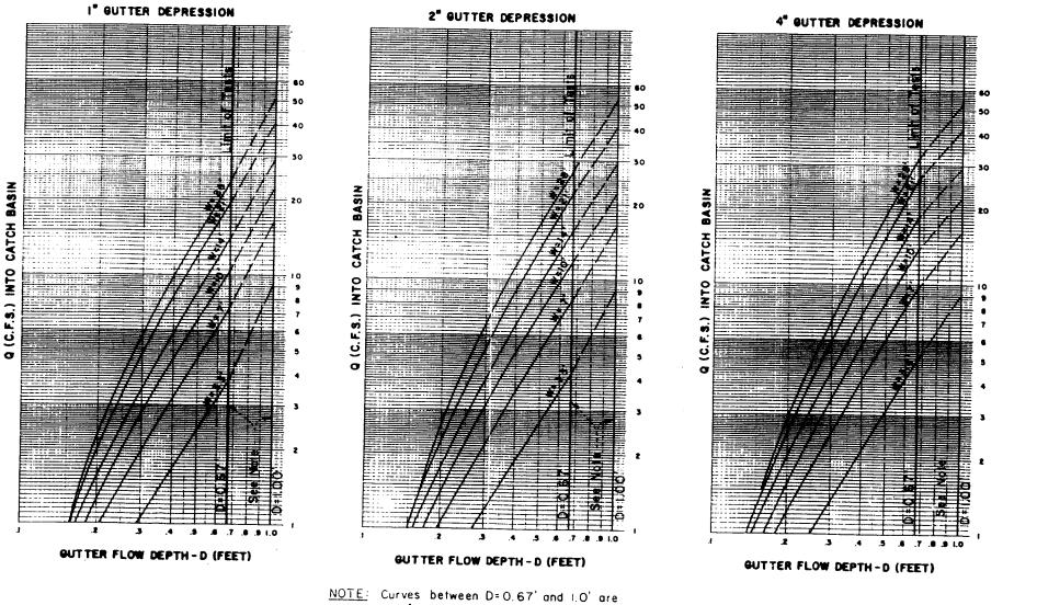
NOTE: Curves between D=0.67' and 1.0' are not from model test data and will be revised in the future when additional model test data are available.
