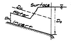
c. Where the water surface of the outlet is below the water surface in the channel or conduit, control will be upstream and the outflow will have the form of a hydraulic drop.
