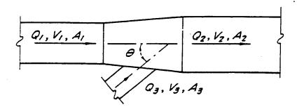
$$\Delta \gamma \cdot A_{\sigma \nu g.} = \frac{Q_2 V_2 - Q_1 V_1 - Q_3 V_3 \cos \theta}{g}$$
