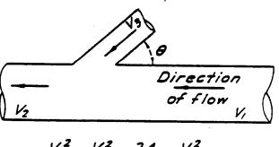
$h_{j} = \frac{V_{2}^{2}}{2q} - \frac{V_{j}^{2}}{2q} - \frac{2A_{3}}{A_{2}} \cdot \frac{V_{3}^{2}}{2q} \cdot \cos \theta$
