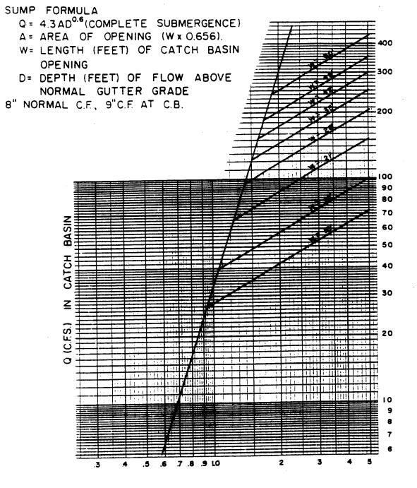
D= DEPTH OF FLOW (FT.) ABOVE NORMAL GUTTER GRADE
