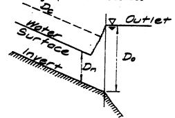
b. If  $P_n+M_n < P_0+M_0$ , this indicates outlet control with a hydraulic jump probably occuring upstream.
