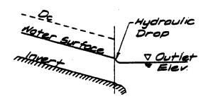
When there is a series of control points, the one located farthest upstream shall be used as a starting point for water surface calculation.
