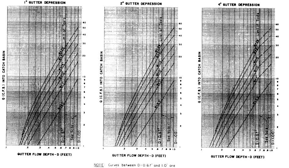
NOTE: Curves between D=0.67' and LO' are not from model test data and will be revised in the future when additional model test data are available.
