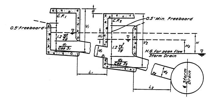
Select a connector pipe size for each catch basin, and determine the related head loss  $(H_1, H_2)$  by means of a culvert equation, or by Chart No. D-30. The sum of head losses in the series shall not exceed the available head, i.e.,
