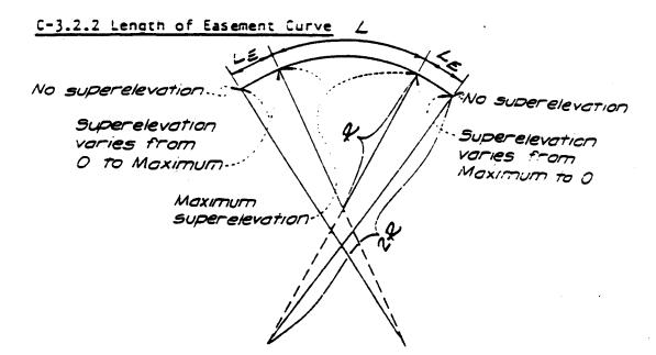
For rectangular channels, the length of easement curve  $(\underline{L}_{\underline{r}})$  is given by the following equation:
